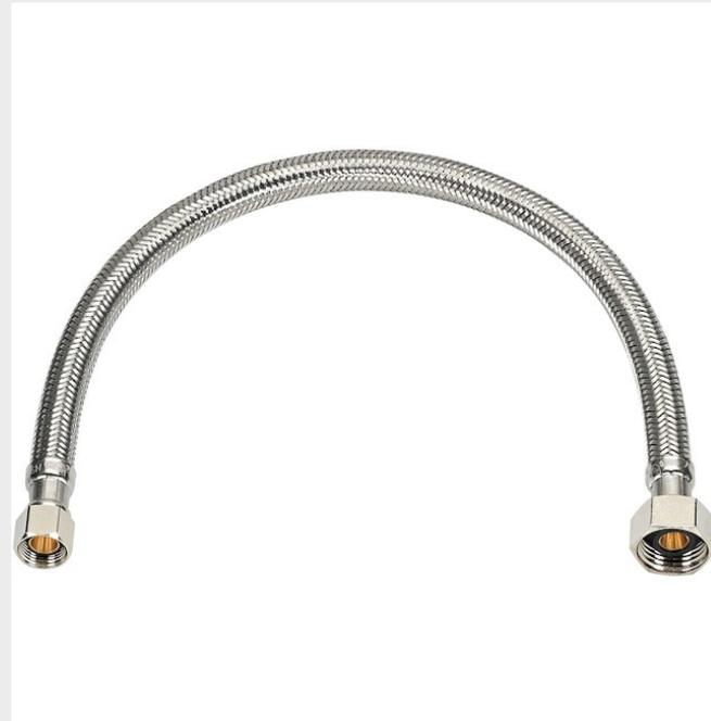
Soft, smooth plastic water lines shall be replaced with approved metallic lines in accordance to the International Plumbing Code. However, hard plastic water lines attached to the shut-off valve **at the factory** are allowable. White braided supply line is acceptable.
