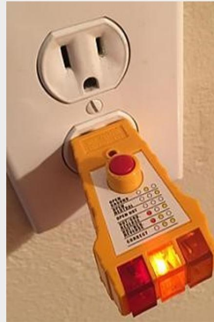
Inspectors check for open grounds and improper wiring with a tester on receptacle outlets. Original two-prong systems are acceptable, if maintained. Three-prong outlets not grounded must be properly grounded, or switched back to two-prong.
